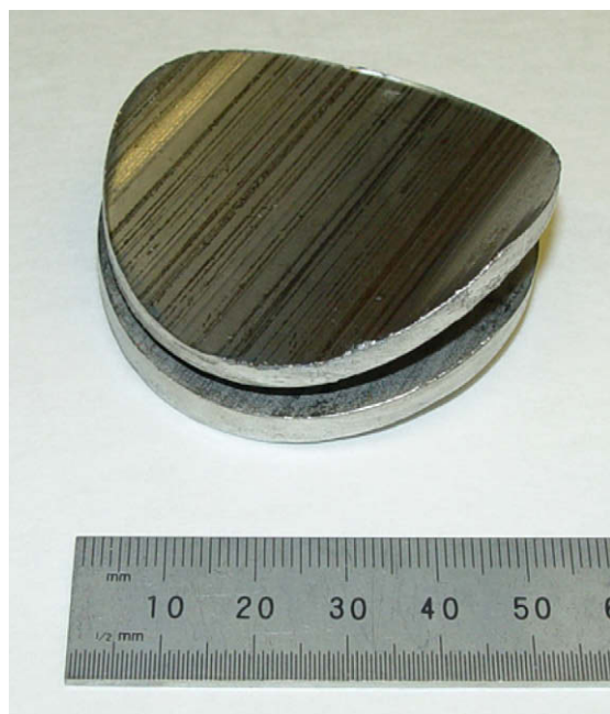
Fig. 7. Example of specimen material obtained with an annular cutter from the nose of a non-irradiated mockup target vessel.
